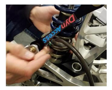
Remove bolt C and the lower shock mount.
