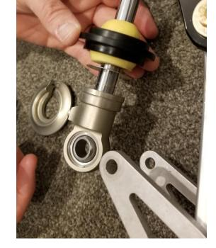
Press up the bump stopper on the shock's shaft approximately 25 mm (1")
