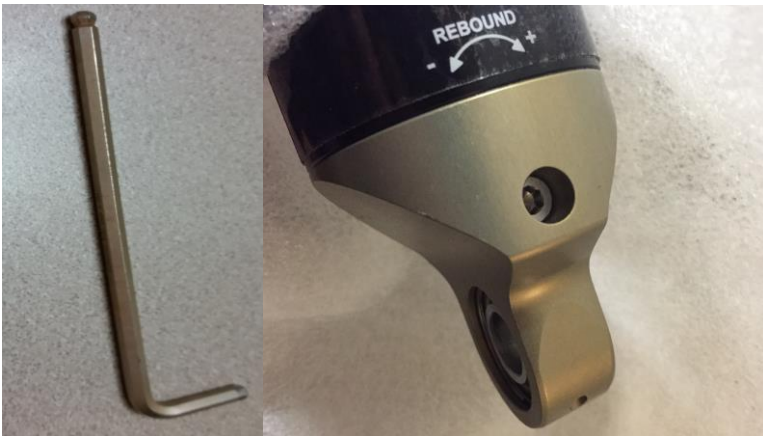
Fig.3. Rebound damping adjuster (needing a 5/32 ball hex wrench)
