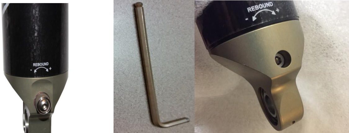
Fig.2. Rebound damping adjuster (Left: knob model, Right: New adjuster, needing a 5/32 ball hex wrench)
